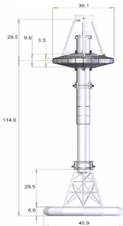
The VWP will use the 'PowerBuoy' wave energy system to extract wave energy and convert to electricity (Figure 2.)
